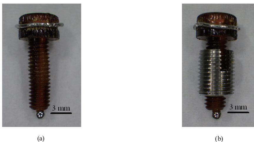
Fig. 1. (Color online) (a) Picture of the recording electrode. The recording electrode had the structure of a plastic screw with a platinum (Pt) ball at the tip. (b) Picture of the recording electrode with threaded insert. The implantation depth of the recording electrode was adjusted via the threaded insert to optimize the recording of VEPs. The Pt ball was placed in a subdural position.
