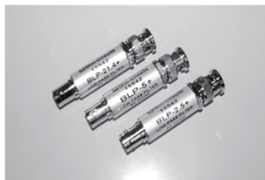
Fig. 1. Experimentally assembled PEA system for thick dielectric materials. (a) Redesigned PEA system, (b) photograph of PEA electrode, and (c) photograph of coaxial low pass filters (BNC type).
